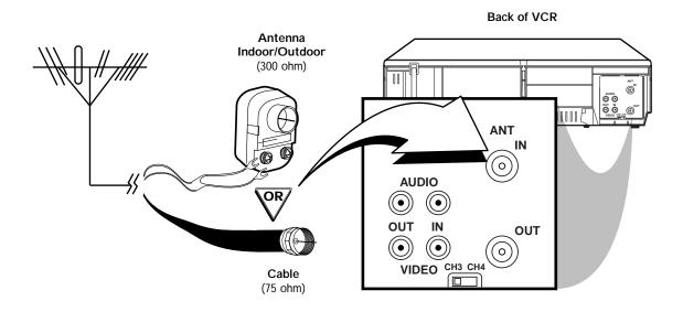
Connect the RF coaxial cable (supplied) to the OUT Jack on the back of the VCR and to the ANTENNA IN Jack on the TV. (You may use either a snap-on type (supplied) or screw-on type of coaxial cable, whichever you prefer.)
